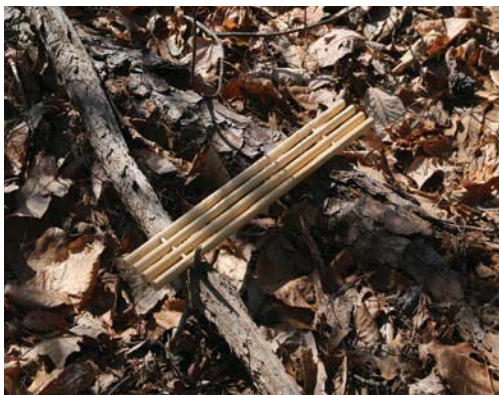
Moisture of 10-hour fuels can be measured with fuel moisture sticks.
