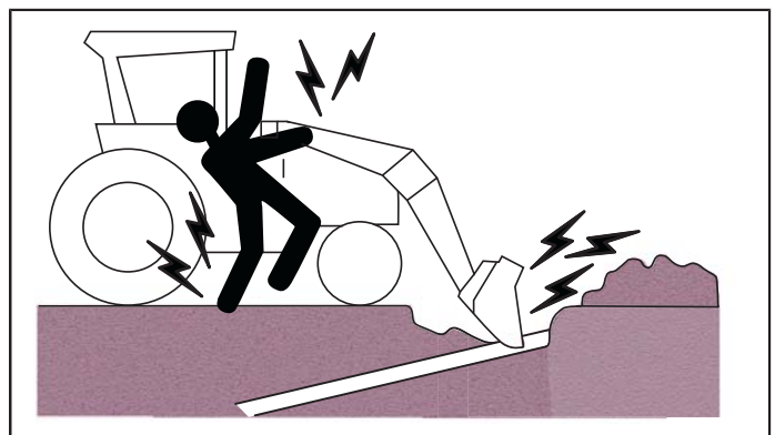
Fig.129 When excavating, make sure there are no hidden electrical cables
