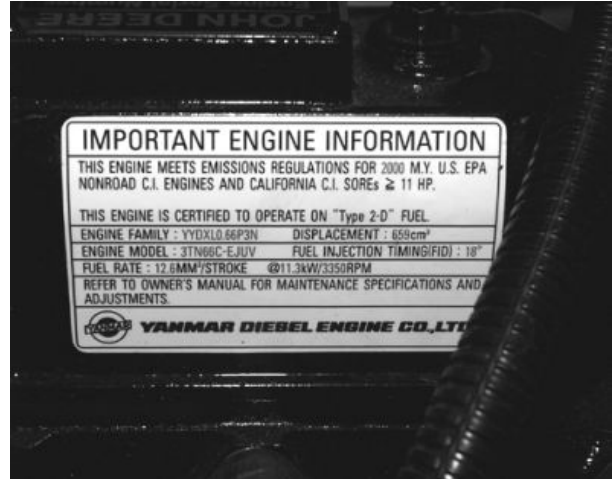
Picture Note: Engine emission compliance sticker located on rocker arm cover.
