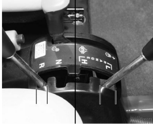
Picture Note: Split picture used to show shift lever centered in both Forward and Reverse positions.
