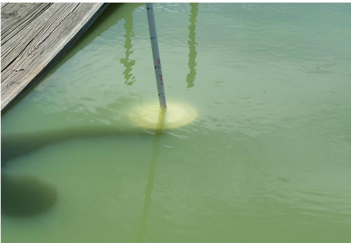
**Figure 6.** Using a white target on a stick to measure light penetration into pond water. The best range of light penetration is between 12 and 18 inches when using a pond fertilization program.
