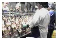
After rehanging, the oil or preen gland is removed from just above the tail and then the birds travel to the evisceration area. During evisceration, a continuous series of machines automatically open the body cavity and remove the viscera, or internal organs. The machines must be properly adjusted so that the cut is carefully made and the viscera are not torn during the proce-
